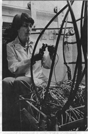
BARBARA STEARNS (5432 - ESA Trainee) works on test setup used to measure effects of radiation on nuclear reactor cabling.
